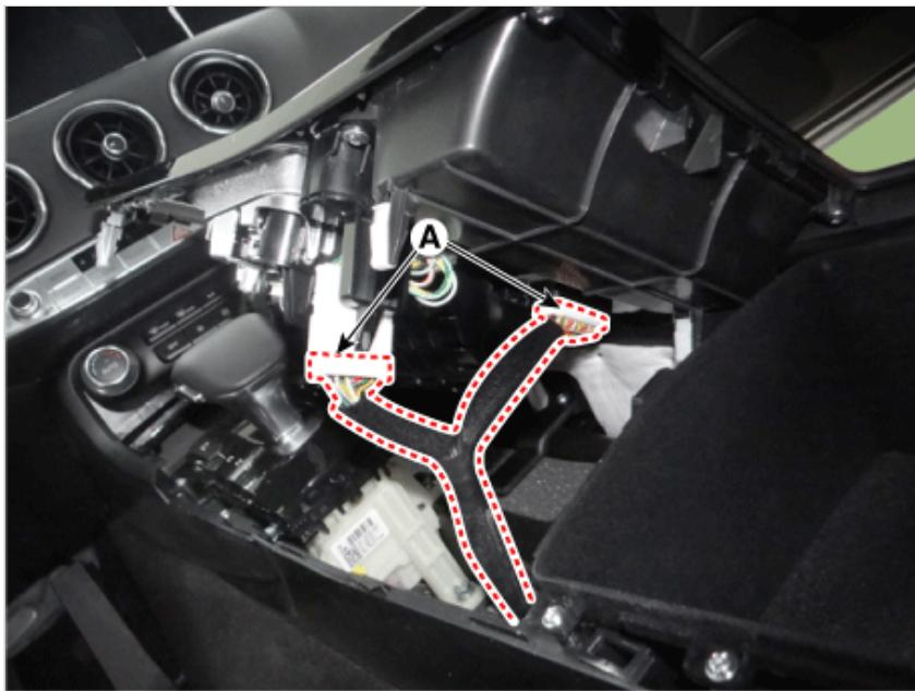
4. Disconnect the connector (A) from the upper console.
