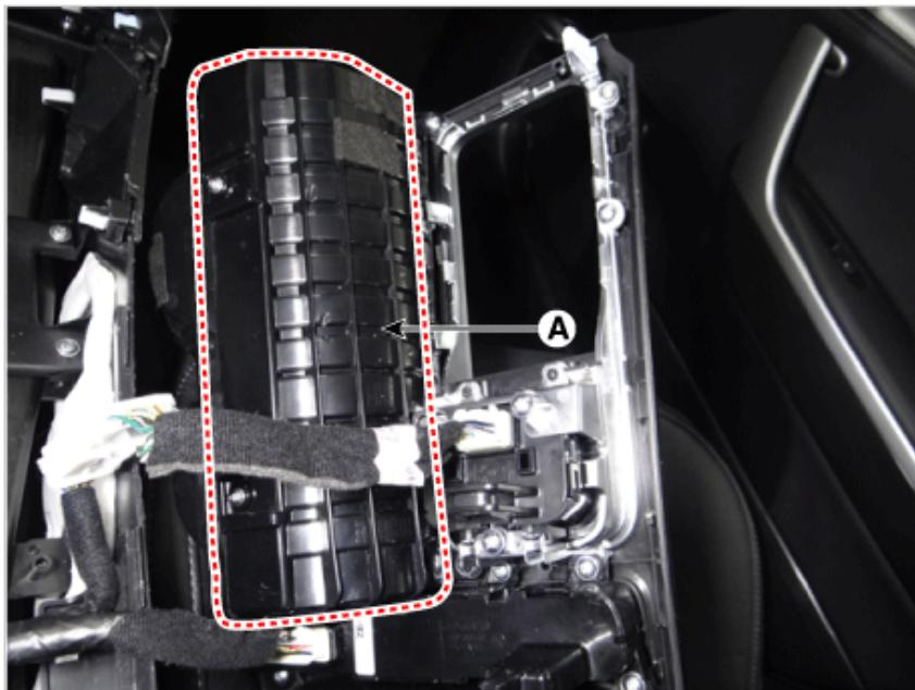
7. Loosen the screw and then remove the ESC switch (A).
