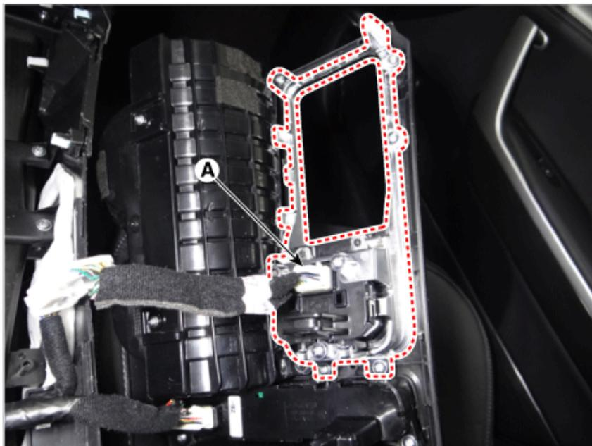
8. Disconnect the ESC connector (A) from the upper console.
